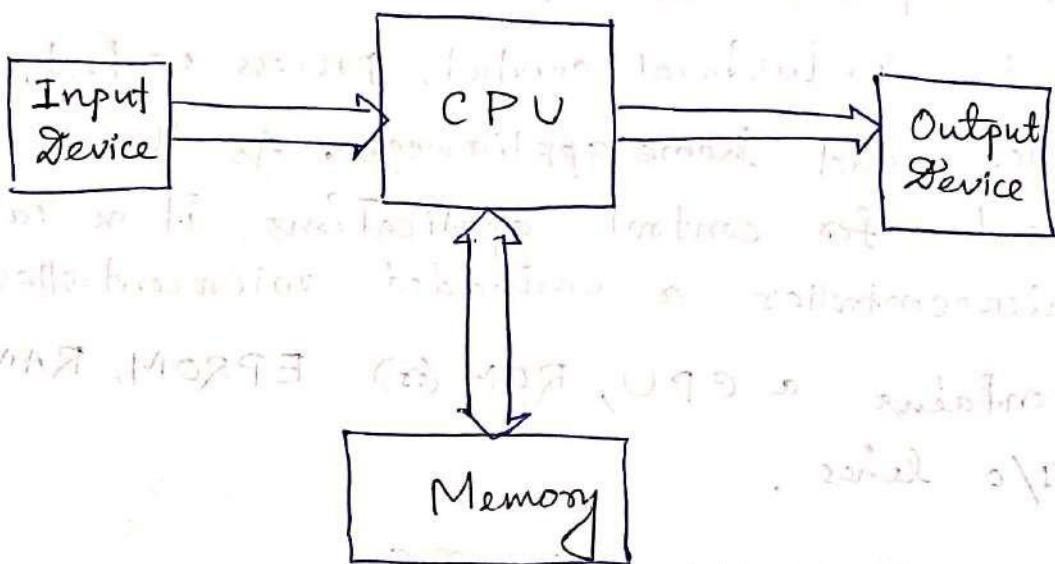
(Schematic diagram of a digital computer)
