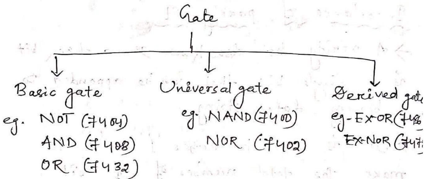
\* EX-OR & EX-NOR gates are available with 2 I/p's only and these gates are 2 I/p controlled gate.
