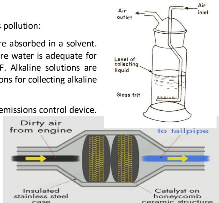
The reduction catalyst is the first stage of the catalytic converter. It uses platinum and rhodium to help reduce the NOx emissions.
