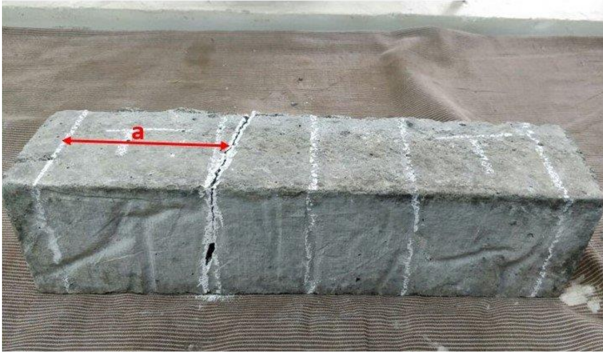
Specimen after Failure for Testing Flexural Strength of Concrete
